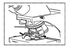
When rotating the nosepiece you must always make sure that the objective which
